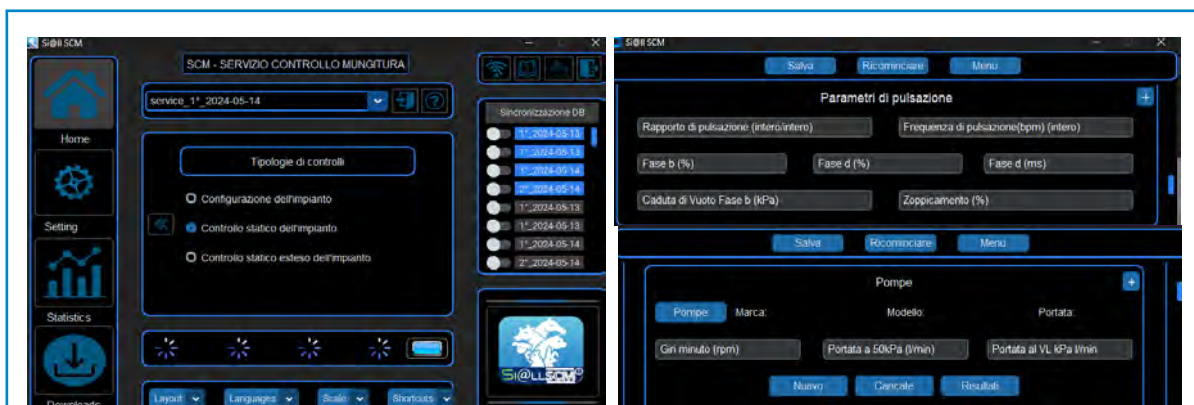
Figure 3. SiallSCM panel to initialize the selected test (left). Data entry mask for pulsation parameters and pump (right).
